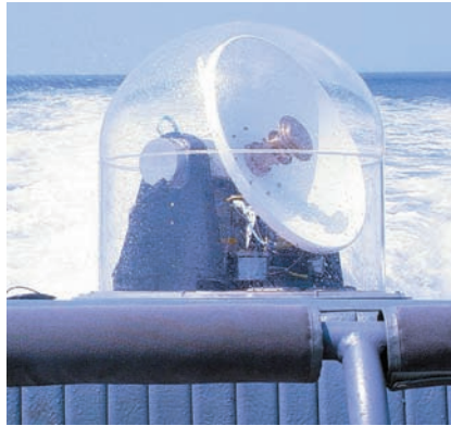
An 18-inch-diameter satellite terminal from DRS Codem acquires an XTAR communications satellite during a Special Operations demonstration. The communications-on-the-move antenna mounted on a Rigid Hull Inflatable Boat can maintain contact with the spacecraft at 20-knot speeds in sea states 2 and 3 with bi-directional datalinks at rates of 3 megabits per second.
