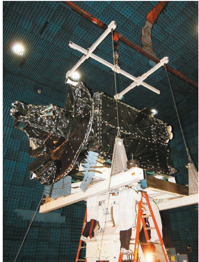
Loral Space and Communications technicians assemble an XTAR X-band commercial satellite prior to launch toward geostationary orbit. The launch, aboard an Ariane 5 ECA rocket from Kourou, French Guiana, provided the second of two powerful, high-bandwidth satellites that form a constellation covering two-thirds of the Earth’s surface with 100-watt, 72-megahertz transponders.
