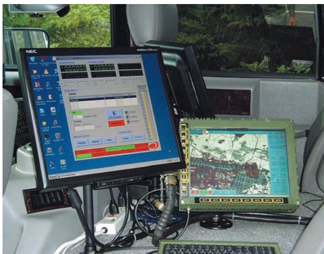
Terminals and equipment mounted in the front compartment of a high-mobility multipurpose wheeled vehicle (HMMWV) display data and imagery from X-band satellites. This DRS Codem ruggedized communications-on-the-move system connects with other mobile platforms—vehicles, ships and aircraft via satellite. An 18-inch-diameter antenna is mounted on the vehicle's roof.
