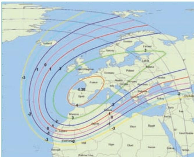
● ● Figure 3: The use of X-band's larger spot beams, combined with bits/Hz efficiencies greater than Ku-band on HTS, allow X-band UAVs higher throughput and a greater operational flexibility than their Ku- and Ka-band counterparts.
