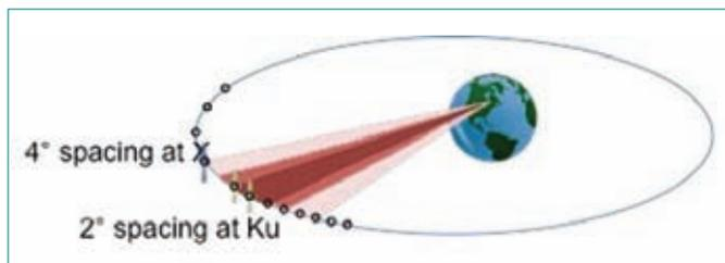
● ● Figure 4: While X-band satellites are spaced at least 4° apart, commercial satellites are typically spaced 2° apart. This difference in spacing allows X-band terminals to operate at higher, more efficient spectral densities. Higher spectral power densities allow small, X-band antennas to transmit at greater efficiencies and throughput – even 2.5x greater than Ku-band on HTS.
